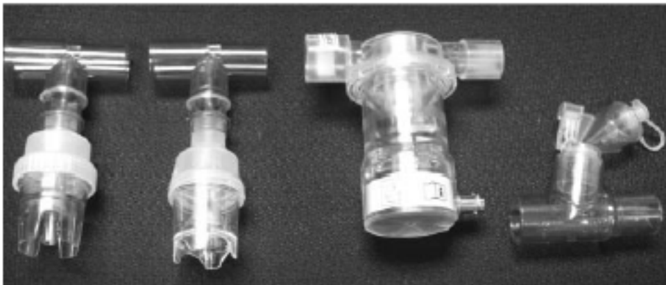
Fig. 1. Nebulizers tested. From right to left: Aerogen Solo, Maquet Ultrasonic model N06302595E400E, Salter 8900, and Hudson Up-draft II Opti-Neb.
